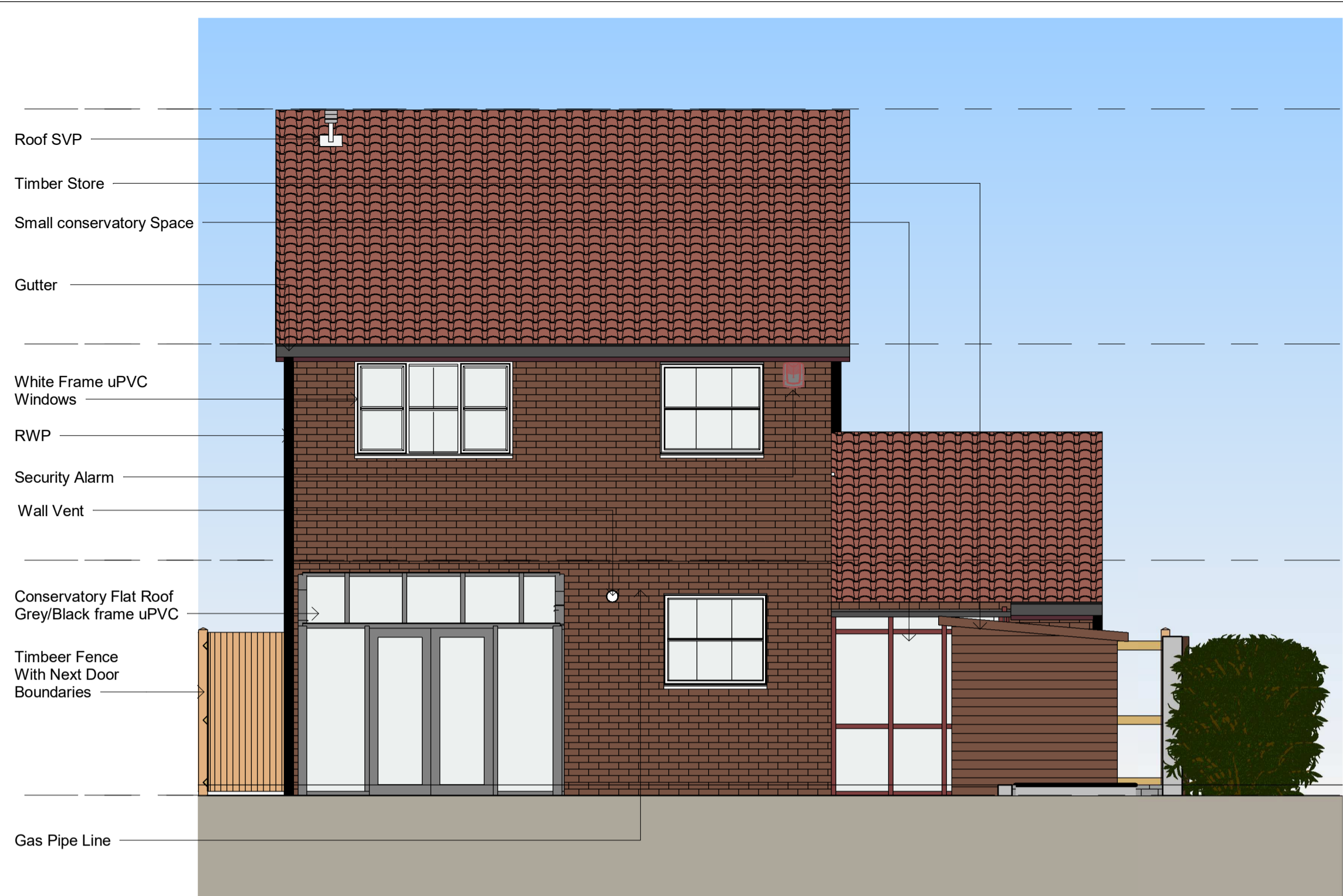
South Elevation (SE) 1 : 50 @A1 1:100 @A3
