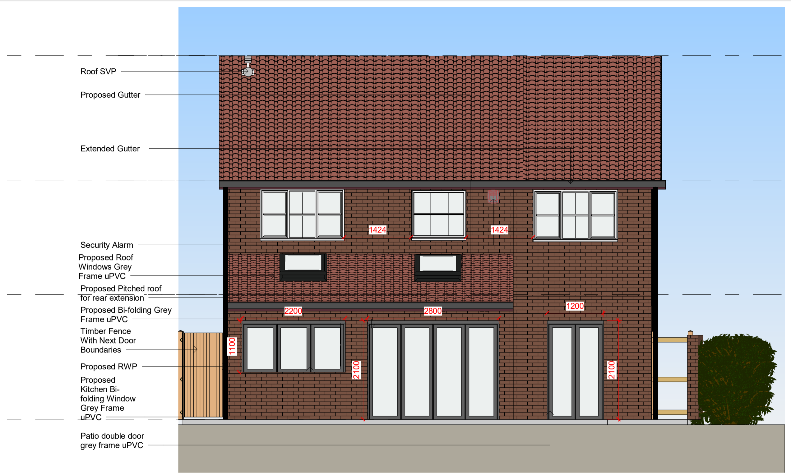
South Elevation_(SE) 1 : 50 @A1 1:100 @A3
