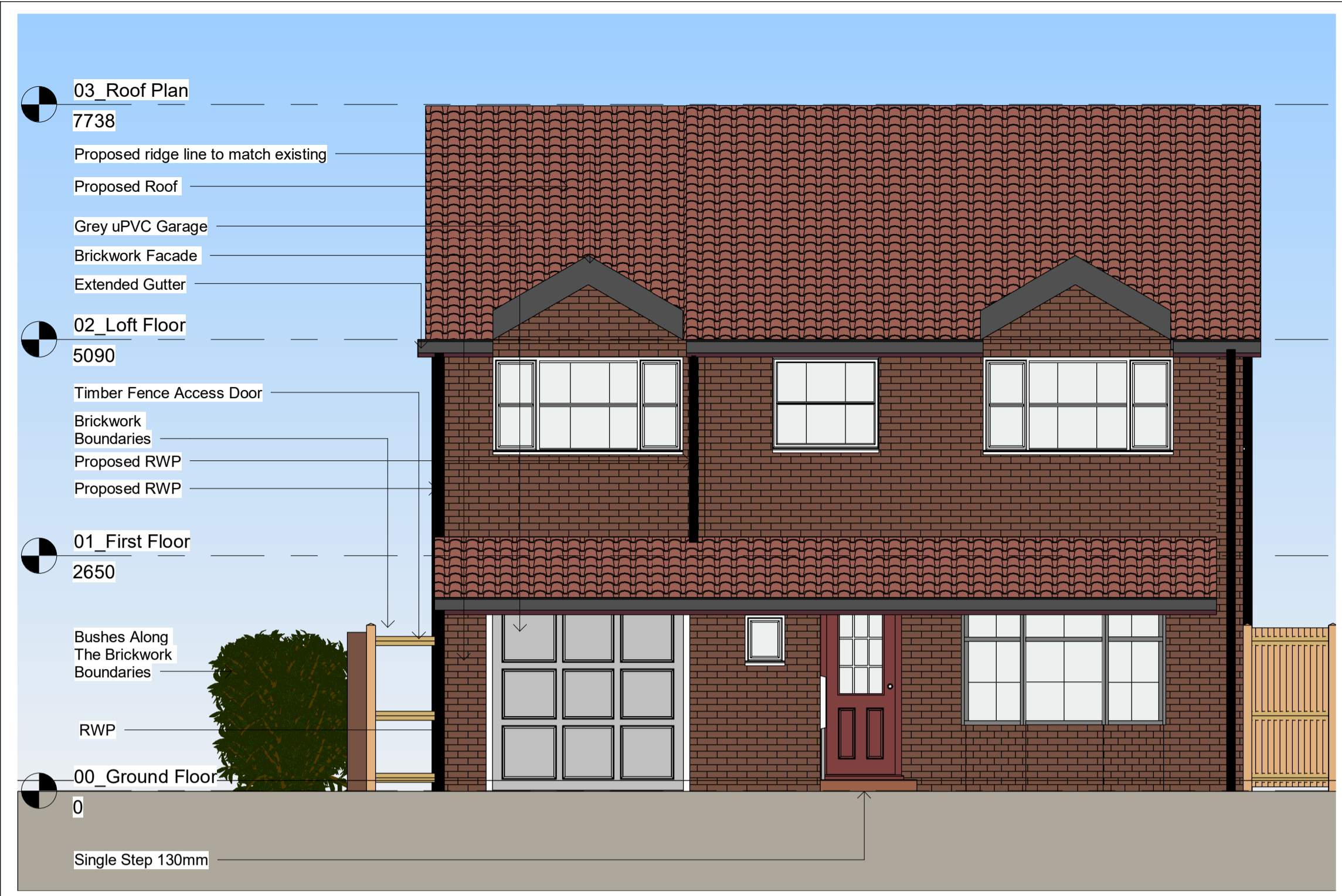
North Elevation_(NE) 1 : 50 @A1 1:100 @A3
