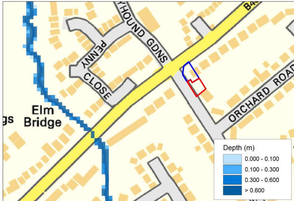
Figure 2-2 Undefended – 1% AEP event modelled flood depths (defended and undefended results are similar in this area)
