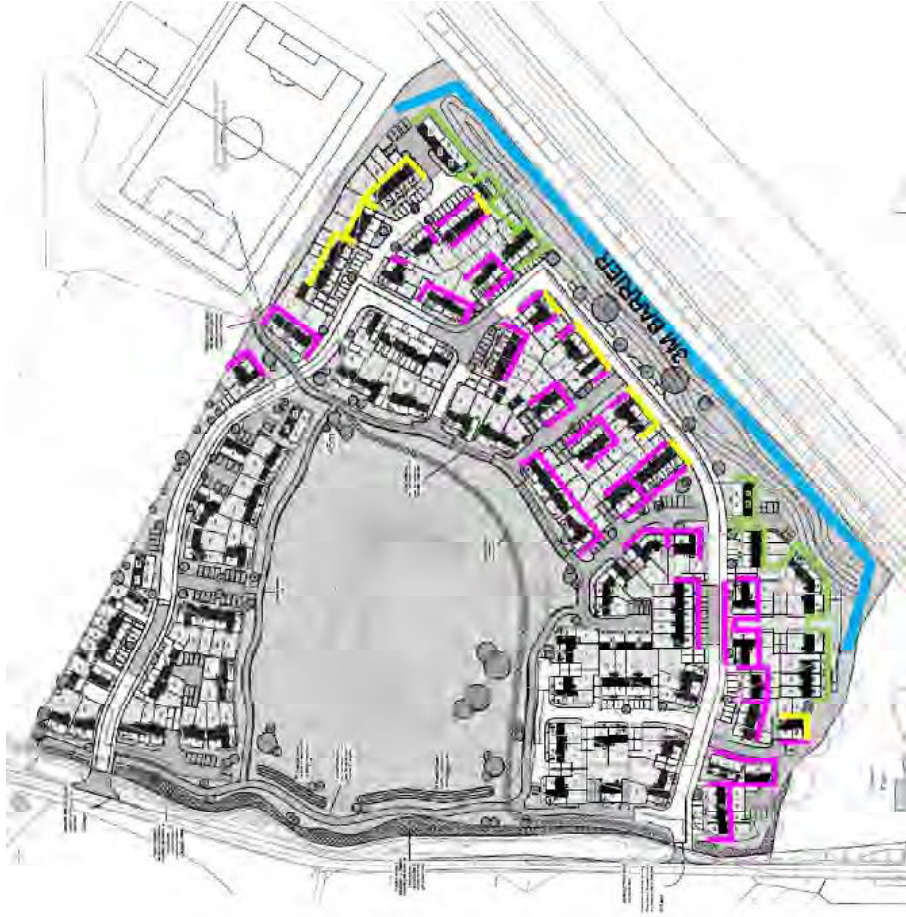
Figure 4.23: Acoustic glazing locations (ref: R9061-1 Rev 1 Land at Snow Capel - Noise Assessment)
