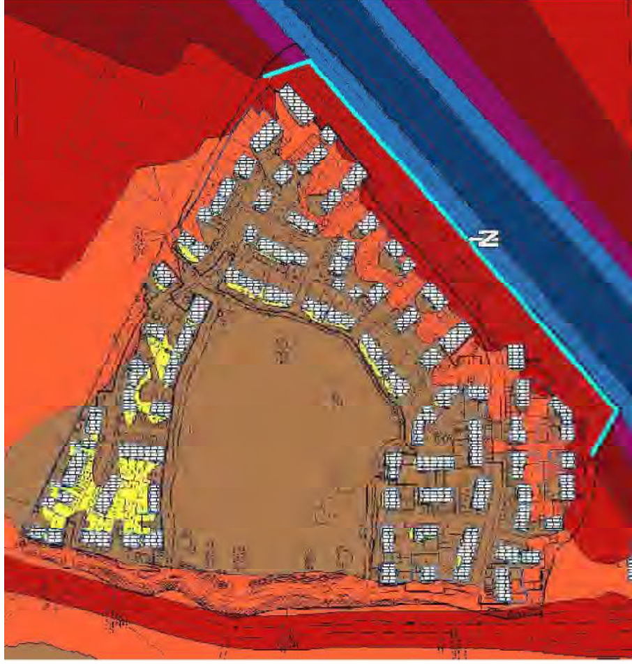
Figure 4.24: Daytime noise contours (ref: R9061-1 Rev 1 Land at Snow Capel - Noise Assessment)
