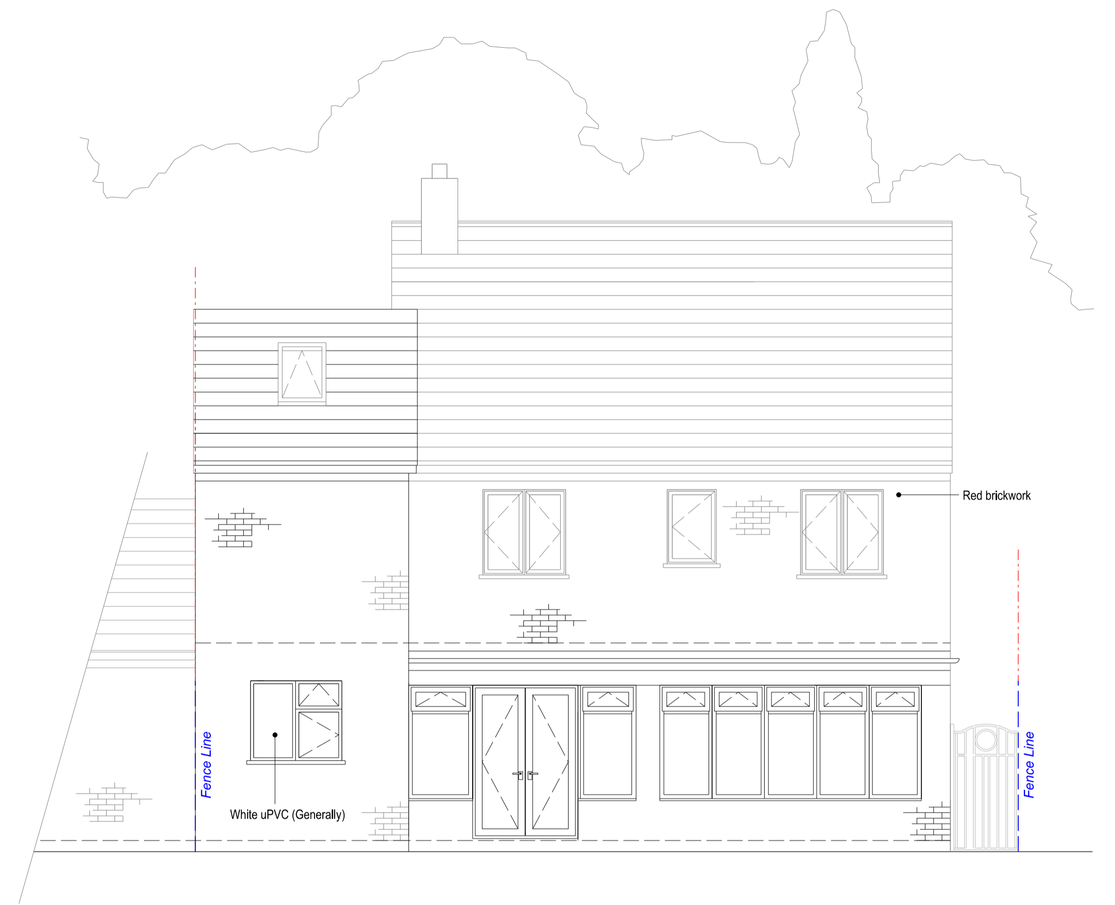
PROPOSED REAR ELEVATION OF PROPERTY
