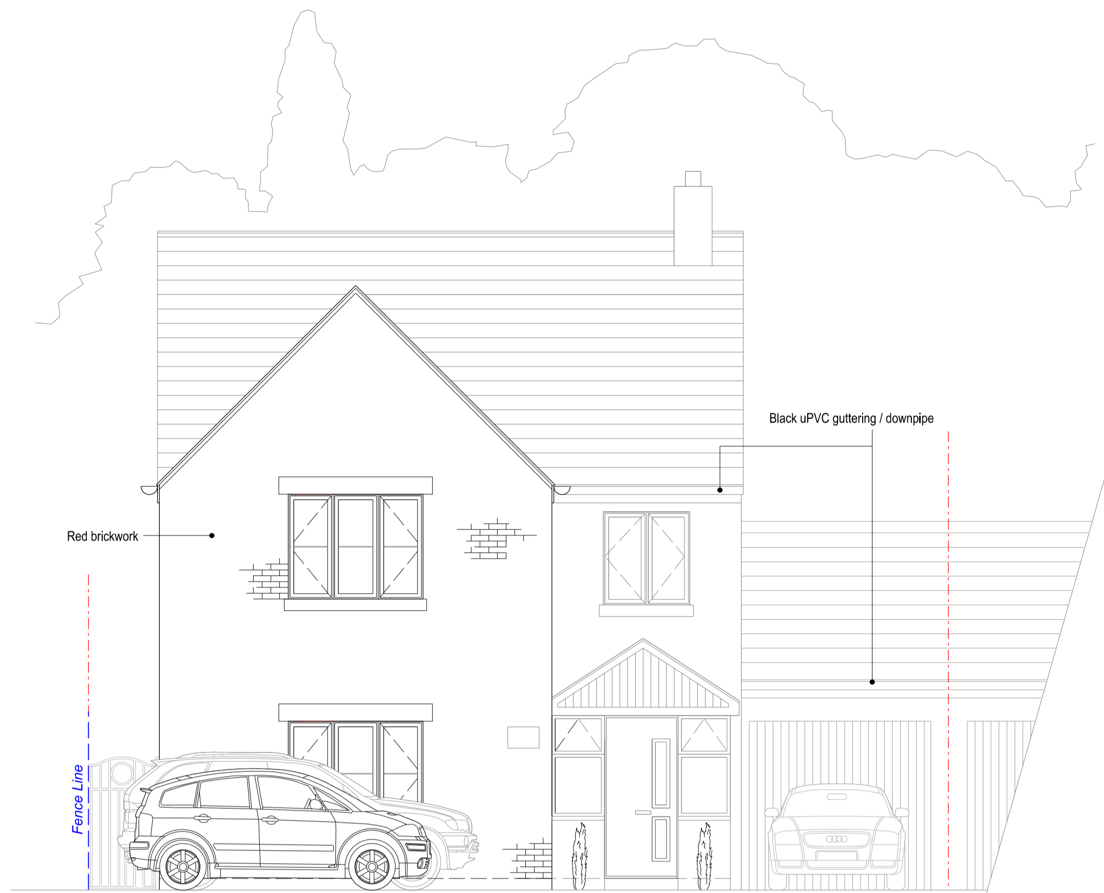
EXISTING FRONT ELEVATION OF PROPERTY
